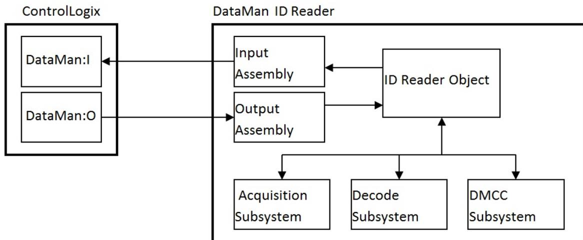
The *Input Assembly* and *Output Assembly* map various attributes (data) from the ID Reader object: The Input Assembly is the collection of DataMan reader data values sent to the PLC (PLC inputs); and the Output Assembly is the collection of data values received by the DataMan reader from the PLC (PLC outputs).
