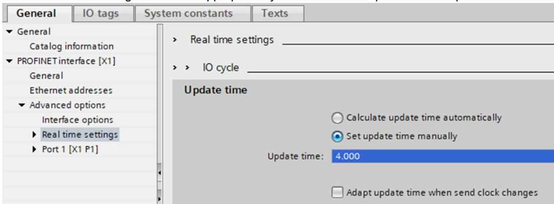
**Note:** The new GSD file has a faster cycle time, defaulting to 4 ms from 8 ms. While this shortens the network update interval, it also doubles the amount of PROFINET traffic from this device.
