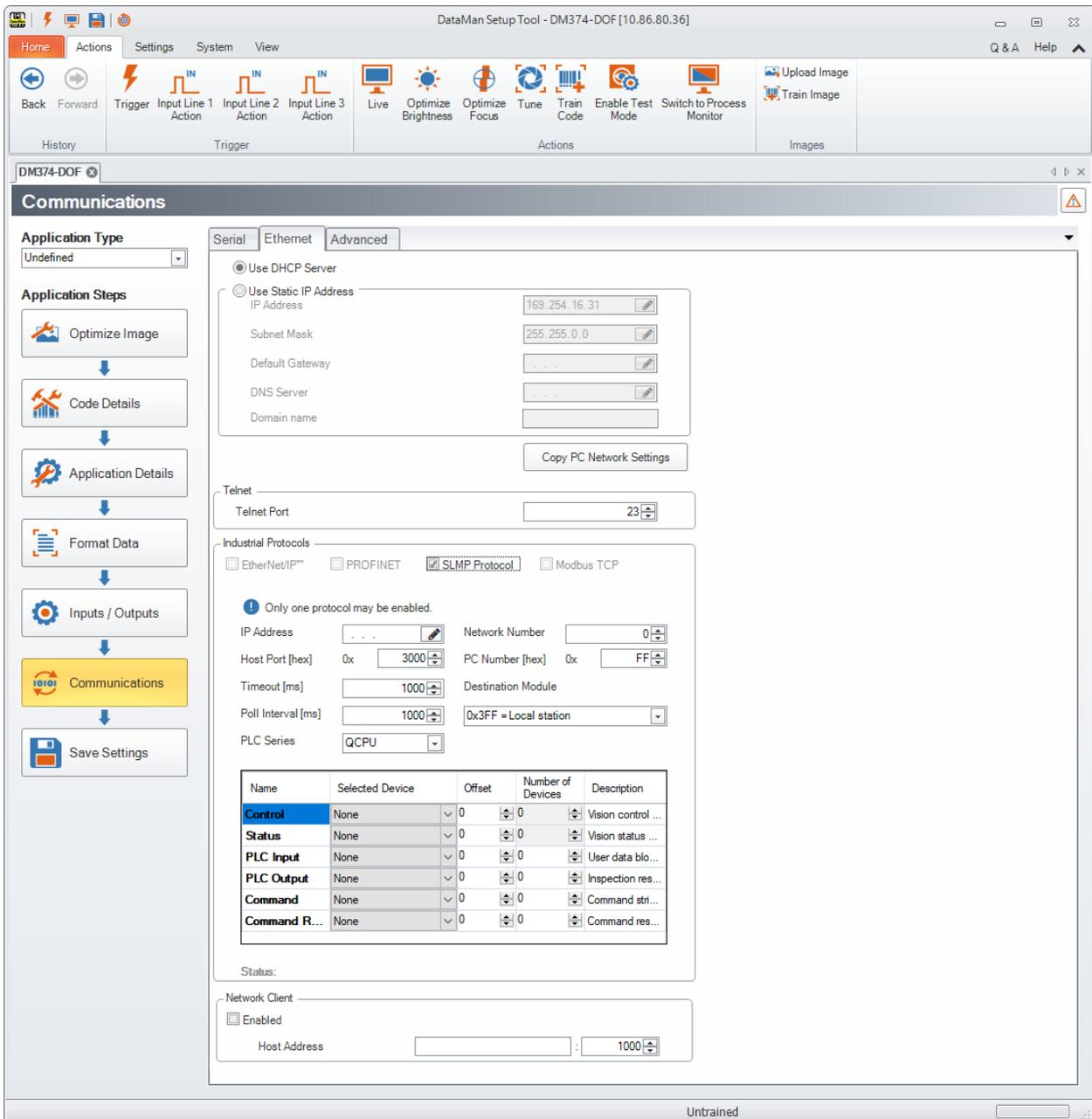
Make sure to save the new selection by clicking the **Save Settings** button in the upper toolbar before disconnecting from the reader.
