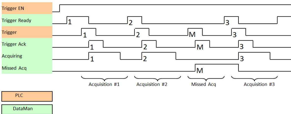
To force a reset of the trigger mechanism, set the *TriggerEnable* to False until *TriggerReady* is also set to False. Then, *TriggerEnable* can be set to True to re-enable acquisition.
