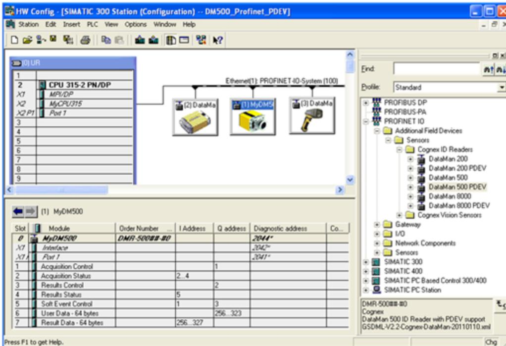
The HW Config tool automatically maps the DataMan I/O modules into the memory space.
