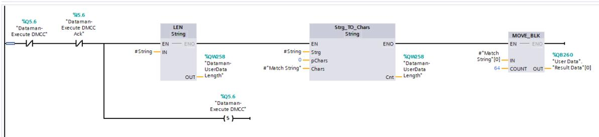
Release "Execute DMCC" signal as soon as it is acknowledged by the reader.
