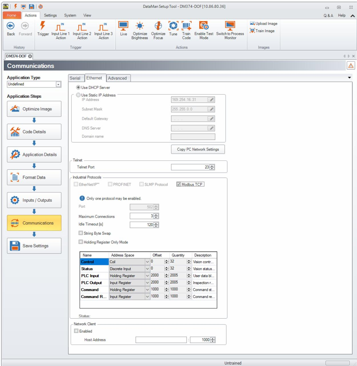
Make sure to save the new selection by clicking the **Save Settings** button in the upper toolbar before disconnecting from the reader.
