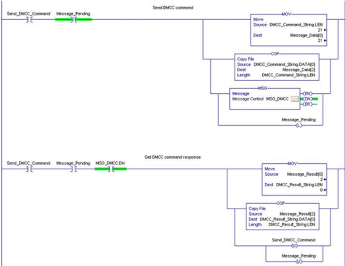
3. Edit the MSG instruction. Configure it for "CIP Generic", service 0x34 "SendDMCC", class 0x79 "ID Reader Object" and instance 1. Set the source to "Message\_Data" and the destination to "Message\_Result".
