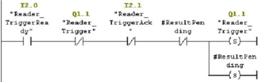
4. As soon as the trigger signal is acknowledged, clear the trigger signal.
