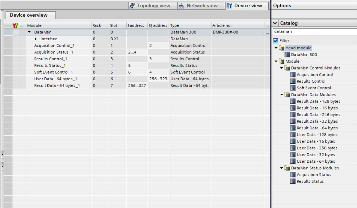
**Note:** Expanding the process image can have a performance impact on the PLC scan cycle time. If your scan time is critical, use the minimal acceptable module sizes and manually remap them down lower in the process image.
