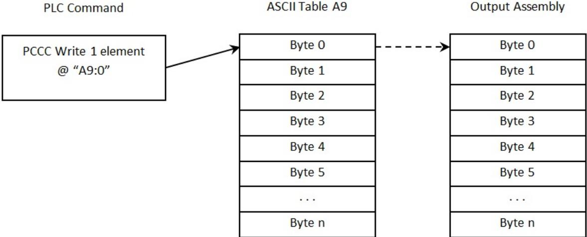
The PCCC Object supports a special case mapping of a string table element (ST10:0) to the DMCC service. Any string written to ST10:0 is passed to the DMCC service for processing. This allows PCCC write string commands to be used to invoke DMCC commands.
