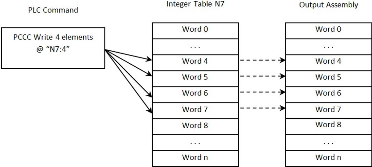
The bit to trigger an acquisition is in byte offset 0 of the Output Assembly. To write to this byte, issue the following PLC command:
