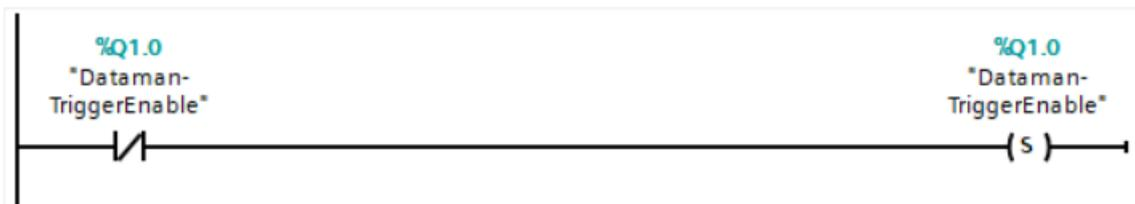
3. Set the trigger signal and set coil to indicate a read is pending.
