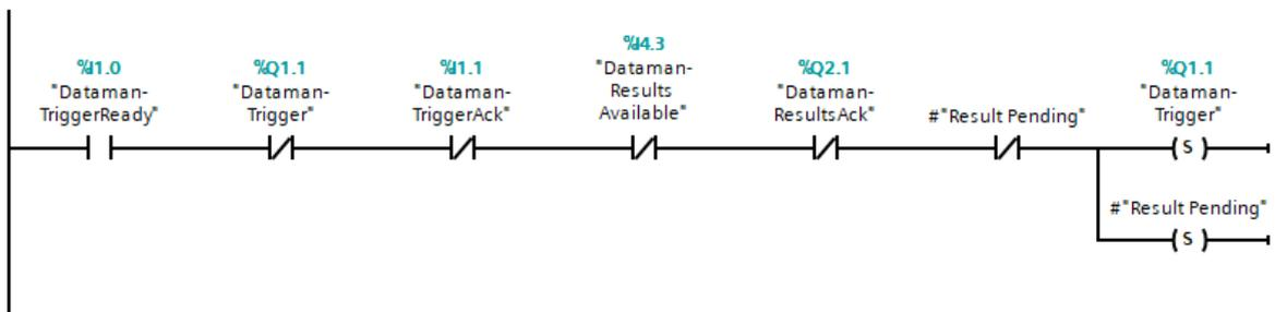
4. As soon as the results are available, clear the trigger signal and save a copy of the result data and set the results acknowledge signal.
