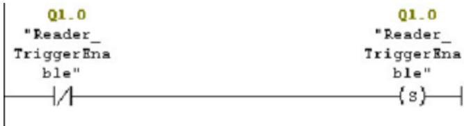
3. Set the trigger signal and set coil to indicate a read is pending.
