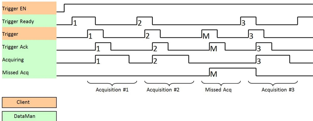
To force a reset of the trigger mechanism, set the AcqTriggerEnable attribute to False until the AcqStatusRegister is 0. Then the AcqTriggerEnable can be set to True to re-enable acquisition.
