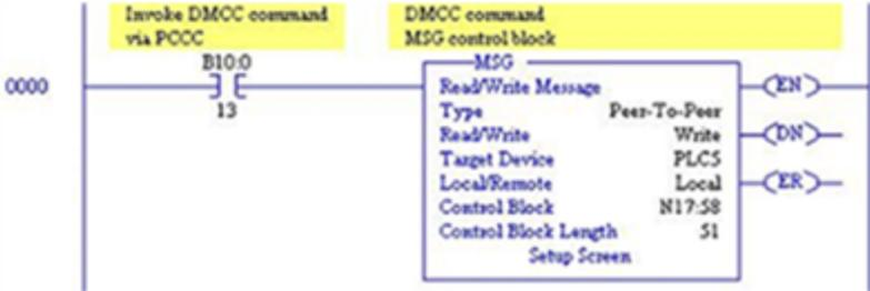
5. Enter the **MSG Setup Screen** and configure it as follows:
