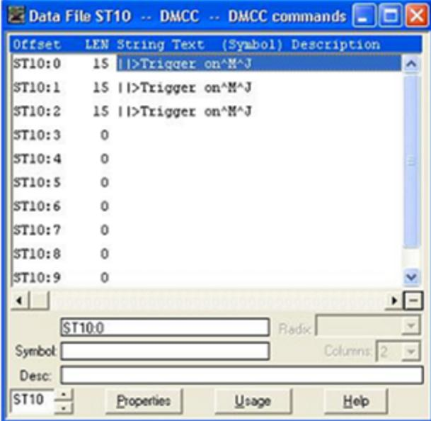
4. Add a new Message (MSG) instruction to your ladder logic and configure it as shown in the following example:
