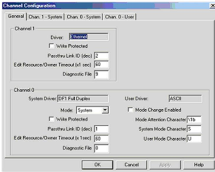
2. The Allen-Bradley SLC has 2 channels available for configuration: Channel 1 (Ethernet); and Channel 0 (DF1 Full Duplex - serial). Click on the **Chan. 1 - System** tab.
