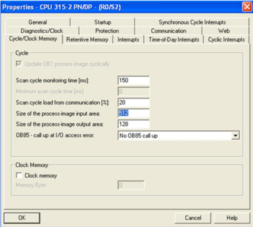
**Note:** Expanding the process image can have a performance impact on the PLC scan cycle time. If your scan time is critical, use the minimal acceptable module sizes and manually remap them down lower in the process image.
